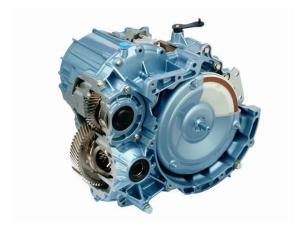
On the drive side, the **Durashift CVT** transmission is equipped with a hydraulic torque converter, which, however is con sequently bypassed by a clutch starting at verv low engine speeds already.
