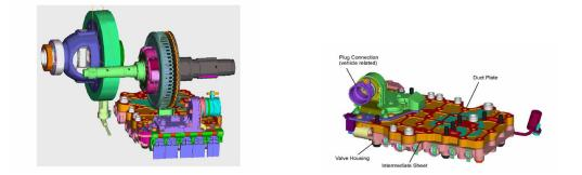
The mechatronic module of the Durashift CVT packages all the control technology in a single control block. Also, there is no wiring harness inside the gearbox.
