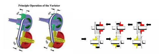
The thrust link belt in Durashift CVT enables seamless selection of gear ratios. The belt and its thrust links are made from high-alloyed maraging steel, originally developed for applications in aerospace technology.
