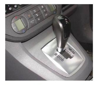
Durashift CVT transmission's gearshift lever can be set for fully automatic selection of the transmission ratios or in the so called select-shift mode when placed in the right-hand shifting slot.
