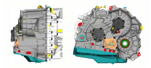
The Ford-ZF CVT in the Focus range is a compact, lightweight unit with a shaft distance of 16.5 cm and a total weight, including the converter and differential, of only 86 kg.
