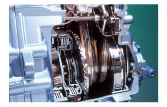
The plantetary gear set responsible for switching between forward and reverse gears is situated on the primary shaft of the Durashift CVT transmission (left), next to it the gear change clutch for the forward-rearward-shifting only and - more to the right - the pair of conical drive wheels for driving the power belt.
