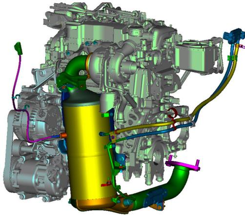
**From the cylinder head to the oil pan, Ford Duratorq TDCi 1.6 is made of aluminium. The particulate filter is located directly below the turbocharger, in front of the engine (viewed in the direction of travel).**
