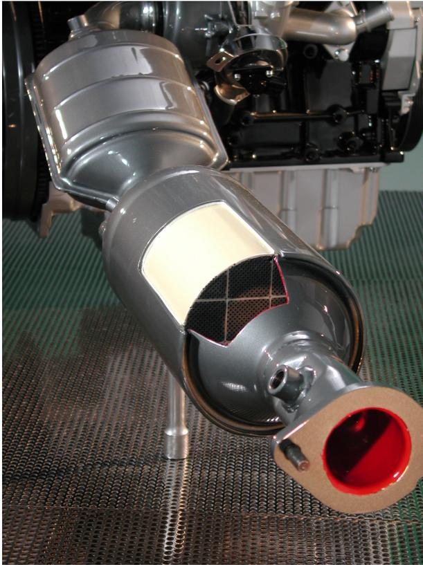
**The diesel particulate trap filter system (dpf) allows the Duratorq TDCi diesel engine of Focus range to operate to the very demanding Euro stage 4 standard. The filter element is located downstream from the catalytic converter and forms a single functional unit with it for regeneration of the particulate filter. The**
