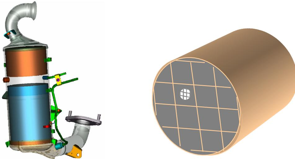
**Complete filter unit as fitted to Ford Duratorq TDCi 1.6 and an individual filter element**
