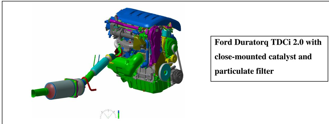
The diesel particulate filter system (DPF) used in Ford Focus and Focus C-MAX fitted with a Duratorq TDCi engine reduces particulate emissions by up to 98 percent and helps to ensure full compliance with the Euro IV emission standard. On the German market, consumers purchasing a Ford Euro IV-compliant diesel vehicle can save up to 614 euros in taxes until the end of 2005 under a government programme promoting the purchase of low-emission vehicles.
