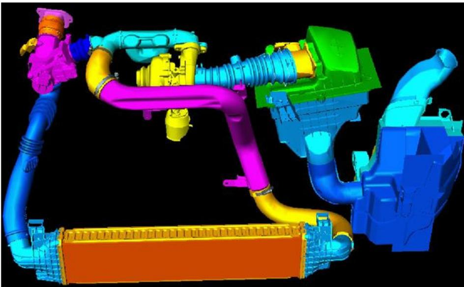
**Characteristic for any Ford Duratorq dpf-filter is the inlet manifold with a split flow function. The reason lies in the fact that for the filter regeneration process to function under low driving load all intake air must bypass the intake air cooler. A split valve, controlling this (top center of the picture) is under control of the motor management system.**
