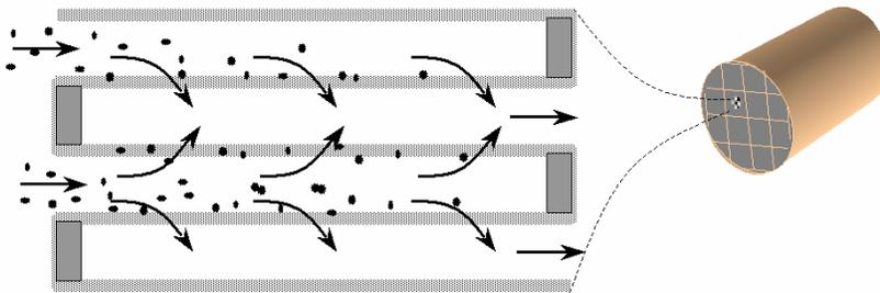
**Ford Duratorq TDCi filter system with filter element made from silicon-**
