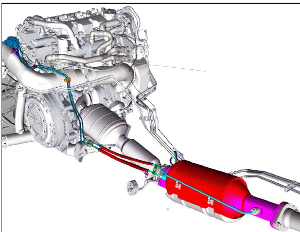
**Ford Duratorq TDCi 2.0 is fitted with a catalyst and particulate filter, designed as two separate components. Viewed in the direction of travel, the catalyst is located behind the engine, close to the turbocharger, the filter roughly below the gearshift lever. This engine uses a**
