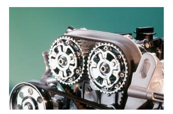
Variable control of both camshafts is performed by two vane-type rotors inside the wheels driving the camshafts. This control is based on a precisely defined programme map and powered exclusively by the engine's
