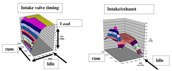
Characteristic of the timing map for the intake camshaft (left) is the fact that, starting at idle (lower right-hand corner), variable timing is passive up to just under 50 percent of the load (yellow field in diagram), then progressively moving towards advance, whereby extremely early intake opening occurs only in the lower engine speed range under full load. The right-hand diagram shows the overlap between both durations, characterised by an extensive range of
