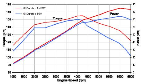
Ford Duratec 1.6 Ti-VCT shows an impressive torque curve over a wide range of engine speeds.
