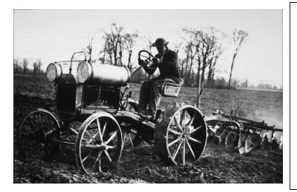
In the good old days of Ford's Model T, engineers had not yet invented maximum engine speed. Instead, the engine's large cubic capacity was fully exploited to develop torque: "Tin Lizzy" delivered impressive 20 hp at 1800 rpm from its 2.89litre displacement, and the veteran's maximum torque of 110 Nm at 900 rpm was not to be sneezed at either.
